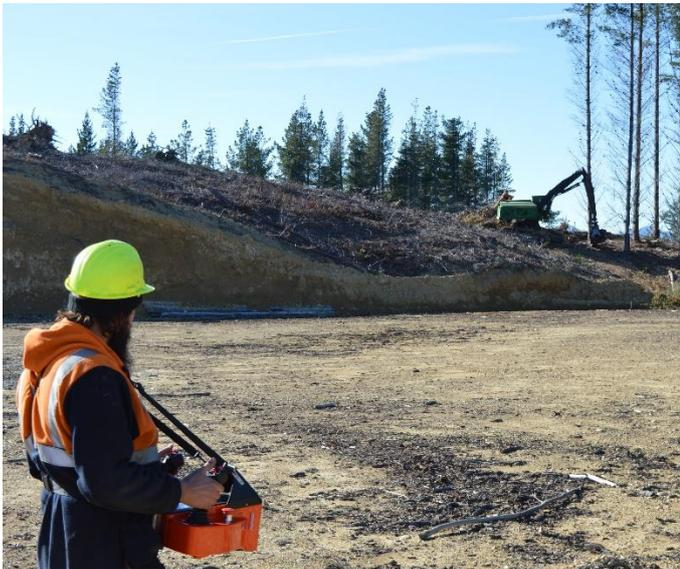
Stage 3 of the project, to implement the full teleoperation system on the John Deere 909 feller buncher that allows the operator to operate the machine from a console (similar to a replica cab) at a distance, using audio and video feedback is now underway. This exciting development for the programme will be achieved in the final year of the programme.
