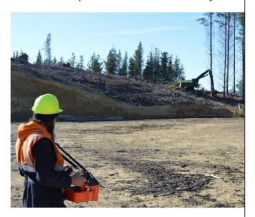
Stage 3 of the project, to implement the full teleoperation system on the John Deere 909 feller buncher that allows the operator to operate the machine from a console (similar to a replica cab) at a distance, using audio and video feedback is now underway. This exciting development for the programme will be achieved in the final year of the programme.
