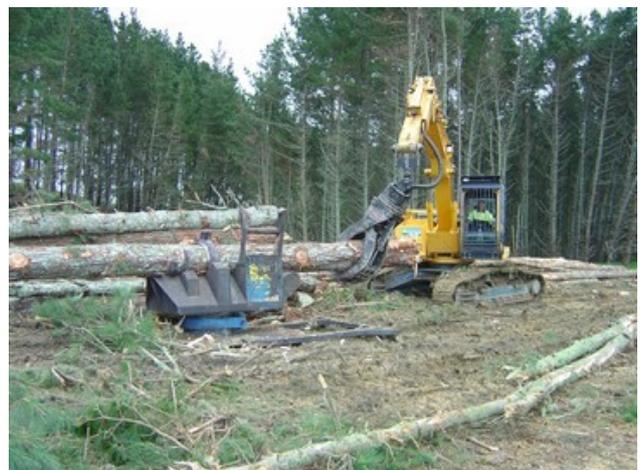
*The static delimiter was evaluated for industry, and its use resulted in significantly fewer branches and other tripping hazards left on the ground. In the study, delimiting time was reduced from an average of 214 seconds per stem to 84 seconds per stem. In addition, logmaker chainsaw sharpening breaks were reduced from one every 29 minutes to one every 53 minutes.*
