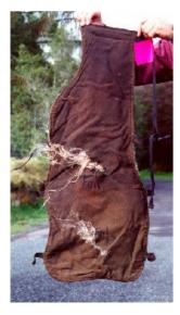
New Zealand research (by LIRA) was used in the development and evaluation of chainsawcut-resistant leg wear. This protective leg wear has dramatically reduced the frequency and of chainsaw severity lacerations to the legs of chainsaw operators.
