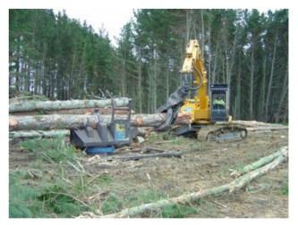
The static delimber was evaluated for industry, and its use resulted in significantly fewer branches and other tripping hazards left on the ground. In the study, delimbing time was reduced from an average of 214 seconds per stem to 84 seconds per stem. In addition, logmaker chainsaw sharpening breaks were reduced from one every 29 minutes to one every 53 minutes.
