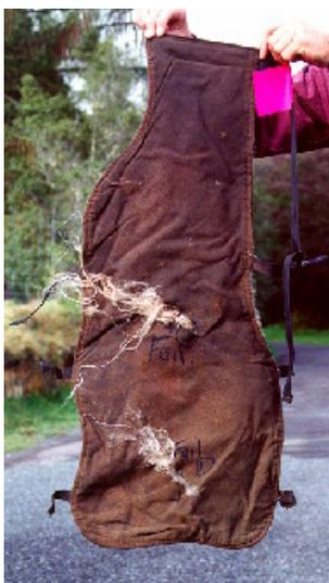
*New Zealand research (by LIRA) was used in the development and evaluation of chainsaw-cut-resistant leg wear. This protective leg wear has dramatically reduced the frequency and severity of chainsaw lacerations to the legs of chainsaw operators.*
