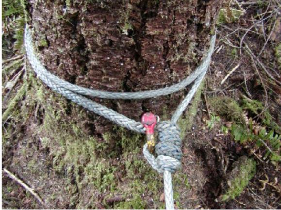
**Figure 2: AmSteel®-Blue synthetic rope used as a guyline (Leonard *et al.* (2003))**
