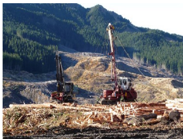
Figure 6: Processor under the Madill tower clearing the chute
