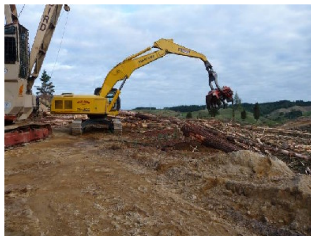
Figure 5: Processor clearing the chute
