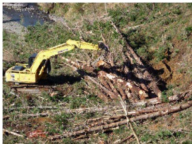
Figure 7: Trees shovelled and bunched for yarder extraction
