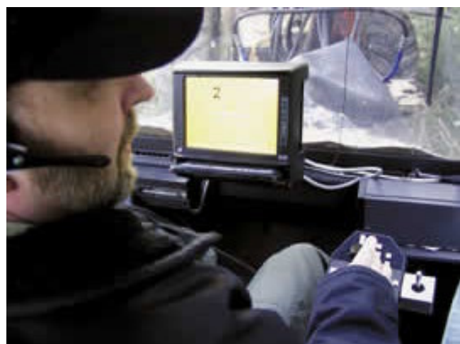
Operator position in the forwarder working with the unmanned harvester
