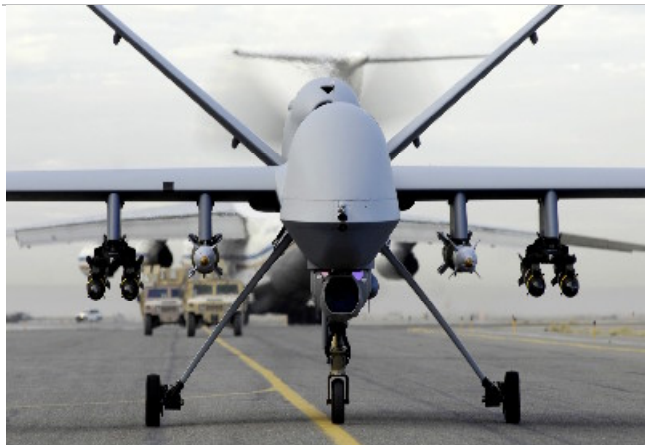
Armed MQ-9 robotic aircraft which is controlled by teleoperation.
