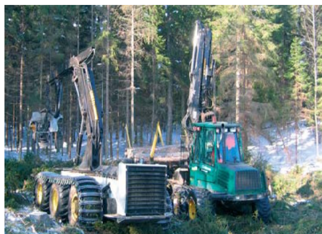
The “Beast” remote controlled harvester (Bergkvist et al. , 2006).
