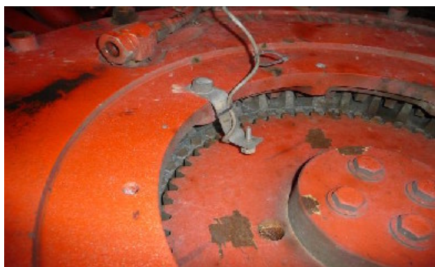
Figure 2. Magnet sensor positions on a drum - drive
