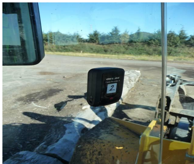
Figure 1: The QSTARZ BT-Q1000XT Travel Recorder positioned on the windscreen of the log loader.
