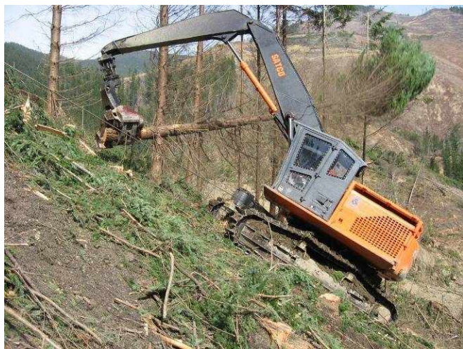
Figure 1. The prototype Kelly-designed steep slope feller buncher
