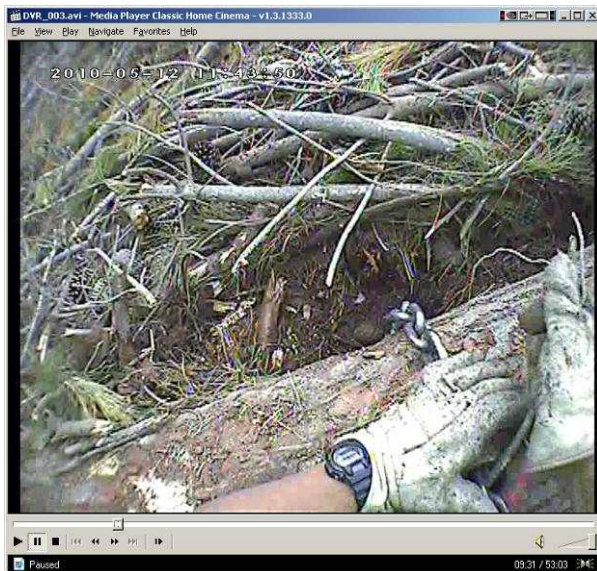
Figure 4: Breaker out hooking on with a chain strop.
