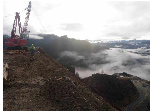
Figure 1: Swing yarder operating in steep country.
