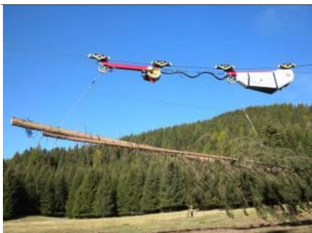
Figure 6: The SEIK 'Sky Bull' two-part carriage showing multiple trees being fully suspended in a horizontal position.
