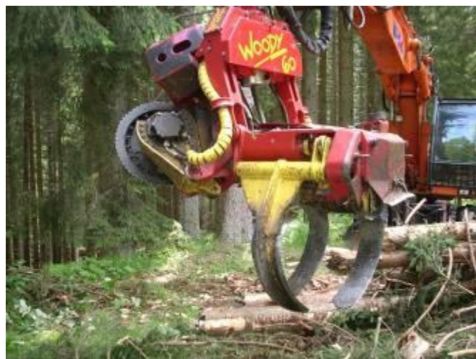
Figure 4: Woody 60 Processor showing the articulated head which allows the knives and rollers to be folded up for improved grapple control.
