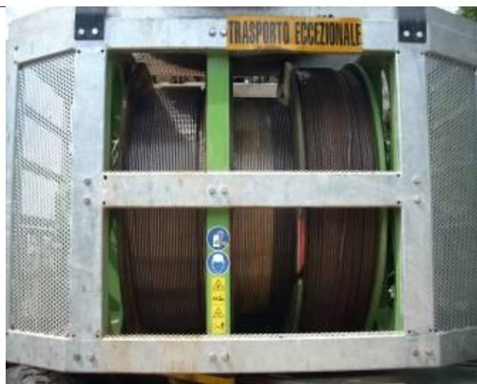
Figure 2: 1500 metres of main rope (on the left) and the 3000 metres of haul back is split between an operating drum and a storage drum. The amount of line in the operating drum is adjusted to the site so that it can turn evenly with the main rope drum.
