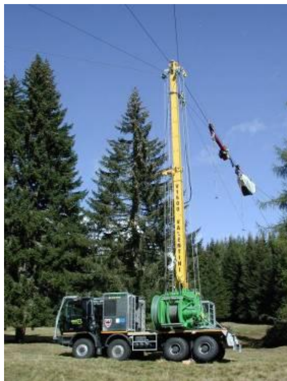
Figure 1: The remote controlled Valentini V-1500 has an 18 m tower, 1500 metres of skyline (3000 m tail rope), main rope speed of 9 m/sec and 7 tonnes of pulling power. One of the most modern yarder designs coming out of Europe, it may find suitability in New Zealand.
