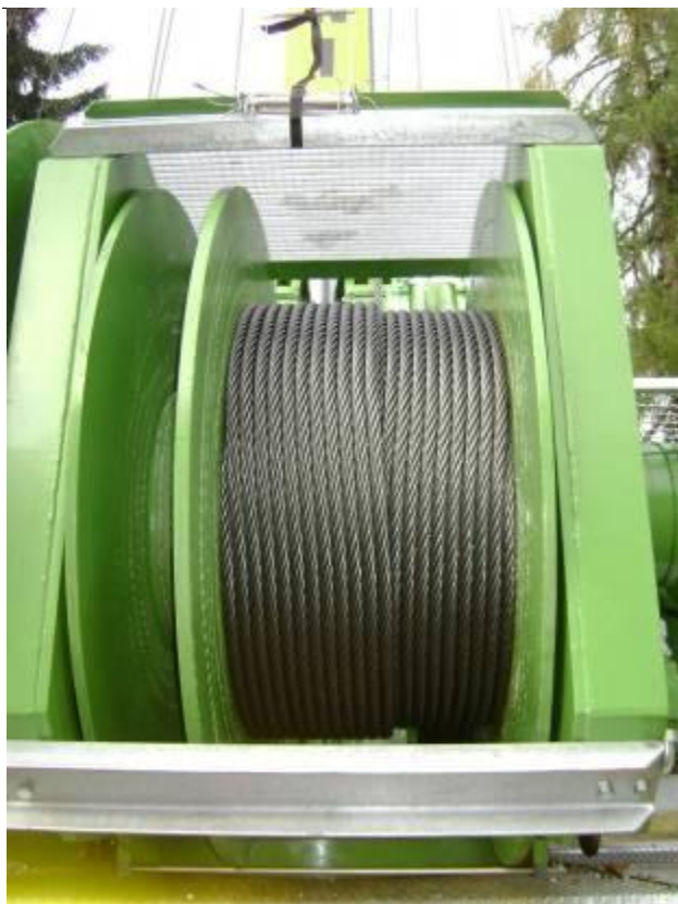
Figure 3: The skyline drum, with the tensioning compartment on the left.
