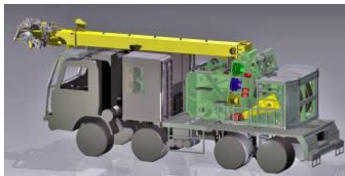
Figure 5: A drawing of the Valentini V-1500 yarder showing the main system components.
