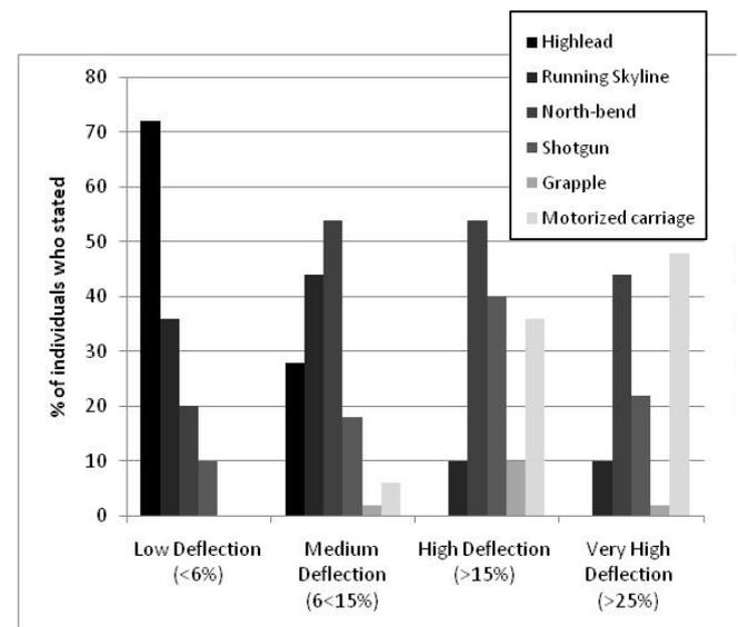
Figure 1: Preferred rigging configuration given percentage deflection.
