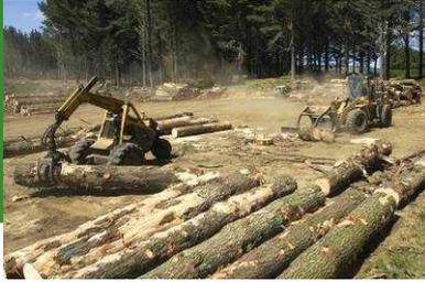
obstacles, and providing full suspension across water courses. Grapples were perceived as being very productive, requiring fewer workers in hazardous roles, therefore being safer to operate.
