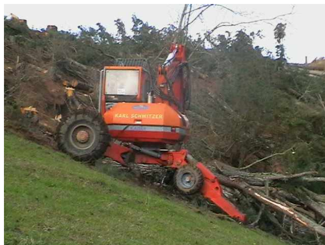
Figure 3: Side view of Kaiser Spyder showing degree of cab levelling possible
