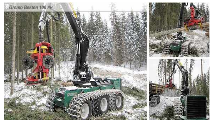
Figure 5: Gremo Besten 106 RH teleoperated harvester in clearfelling in Sweden.
