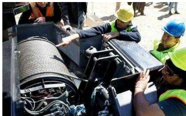
Figure 8: The redesigned winch of the ClimbMax steep slope harvester (Photo courtesy of FICA).
