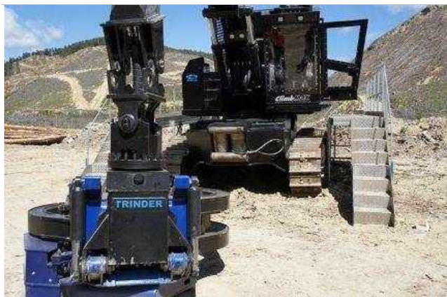
Figure 7: The Beta prototype of Trinder's steep-slope feller buncher featuring Trinder-designed felling grapple (Photo courtesy of FICA)
