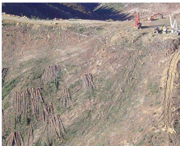
Figure 6: Bunched wood ready for grapple yarder extraction.
