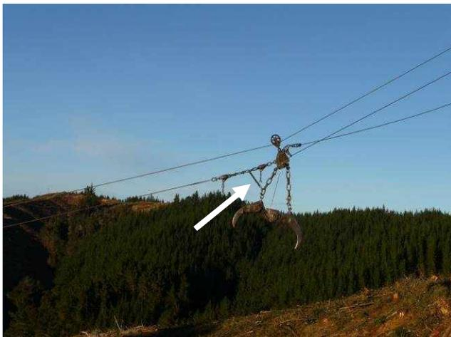
**Figure 2: A simple chain restraint, holding the tines in a desired position for grappling bunched wood**
