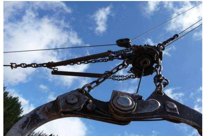
**Figure 9: The Mark 4 Prototype grapple restraint fitted during the field evaluation**
