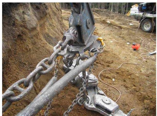
**Figure 6: The Version 3 restraint, showing the attachment to the grapple itself**
