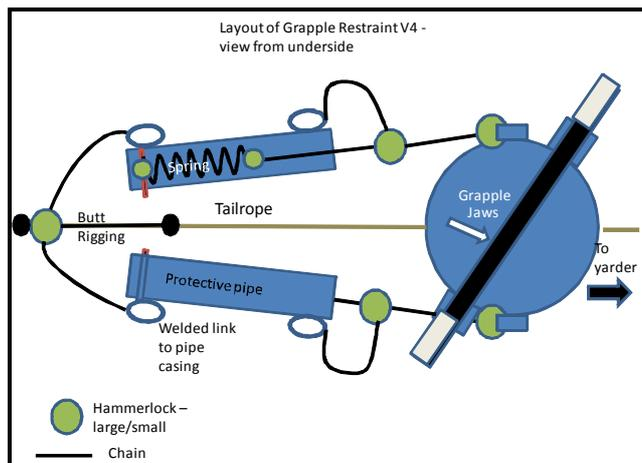
**Figure 8: The layout of the prototype grapple restraint system (V4)**
