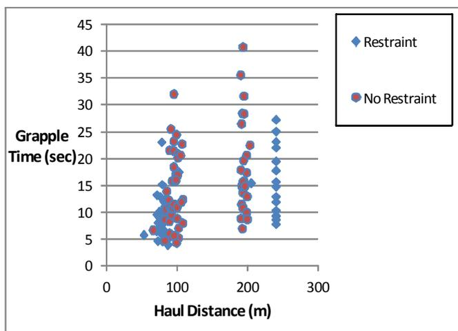
**Figure 13: Grapple time vs. haul distance, with and without the use of the restraint**
