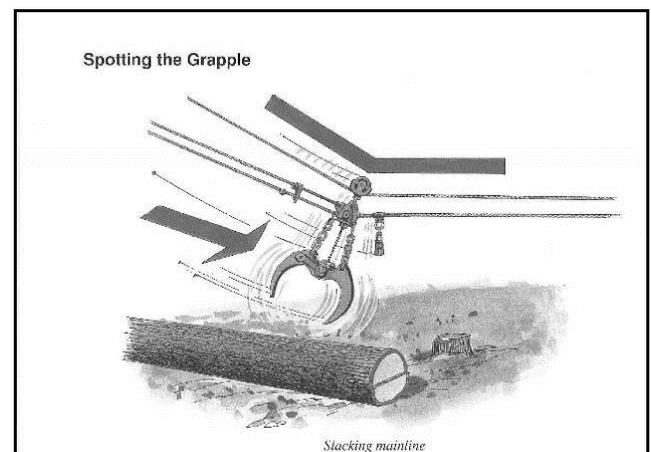
**Figure 1: Spotting the grapple by slacking mainline to move grapple towards tail hold (Ref: WCB of British Columbia)<sup>[1]</sup>**
