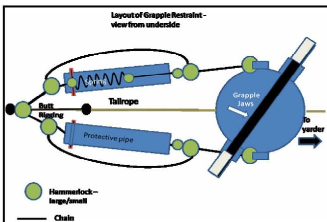
**Figure 4: The layout of the prototype grapple restraint system (V3)**
