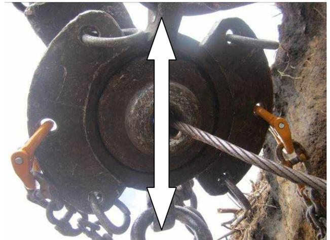
**Figure 5: The location of the attached plates. The hammerlocks are attached so the grapple tines (arrows) are parallel to the ropes**
