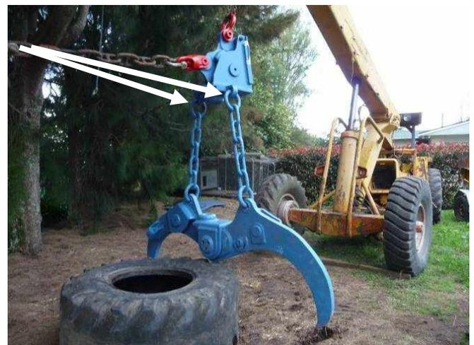
**Figure 3: The Micron grapple used for testing. Arrows show the grapple attachment point to the haul back rigging and control principle for the prototype restraint system**
