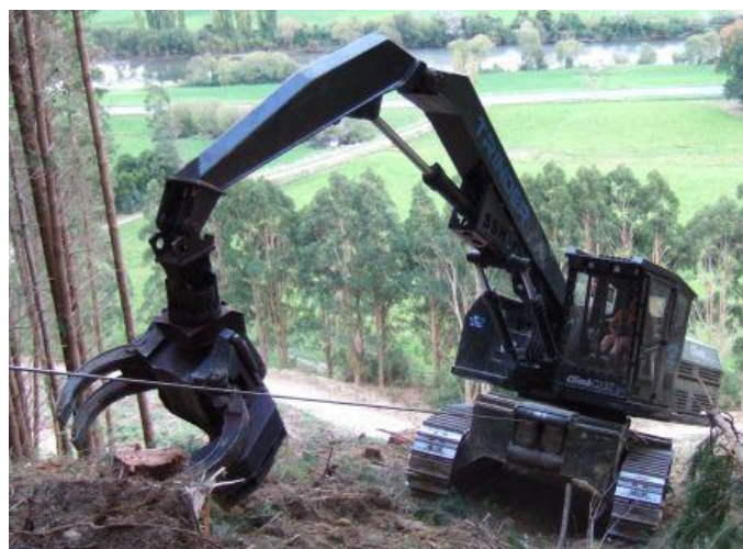
Figure 1: The beta prototype ClimbiMAX Steep Slope Harvester operating in Nelson.
