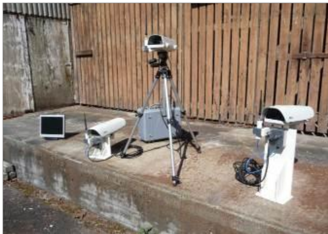
Figure 2: The Hauler Vision System showing (from left): Display, Tailhold camera, Tripod-mounted cutover camera and hauler-mounted camera.
