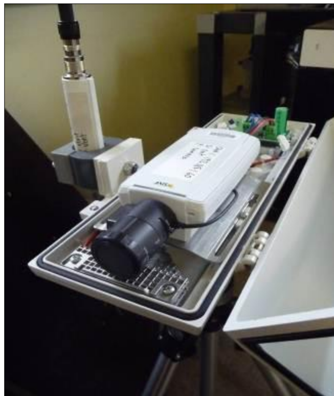
Figure 1: The tripod-mounted camera in position in its protective housing.
