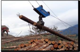
Figure 1: Forestry Falcon Claw, Prototype 3.
