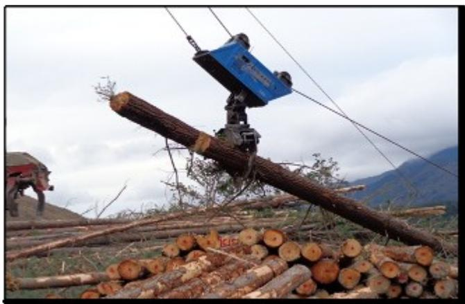
Figure 1: Forestry Falcon Claw, Prototype 3.
