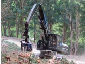
Figure 2: ClimbMAX1 Steep Slope Harvester.
