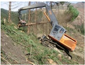
Figure 1: Prototype Steep Slope Harvester (Trinder Engineering).
