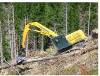
Figure 3: ClimbMAX2 Steep Slope Harvester (Hyundai carrier).
