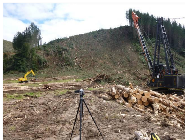
Figure 3: Downhill yarding with the Alpine Grapple
