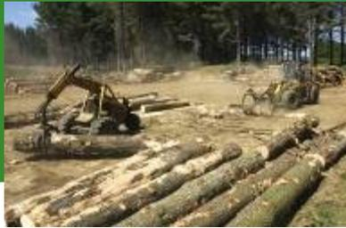
for forestry work, raising the chassis clearance, modifications of engine and hydraulics to suit steep terrain, lengthening the base for extra stability, and an integrated control system to operate the winch. A blade at the back can be lowered to stabilise the machine on steep slopes if required. With the cable being winched in from the machine, the cable is not being dragged over the ground. It is secured at the top of the slope using a stump, “deadman” anchor or mobile anchor.
