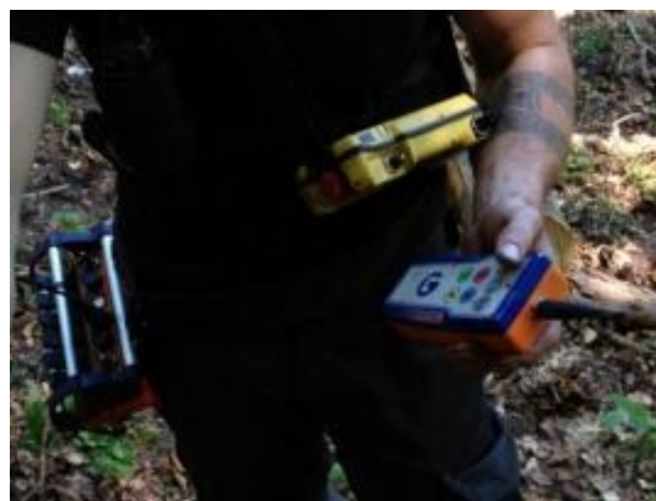
Figure 5: Hauler remote control (left) carriage remote control (centre) and self-releasing choker control (right).
