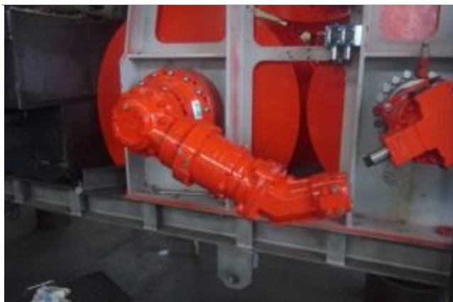
Figure 2: Hydraulic motor, brake and planetary system
