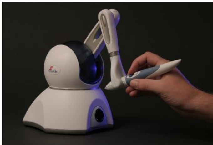
Figure 2: Sensable Technologies 'Phantom Omni' controller which provides haptic feedback
