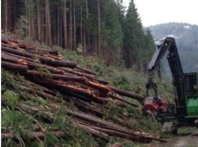
**Figure 4: Mechanical processing of decked wood at roadside**
