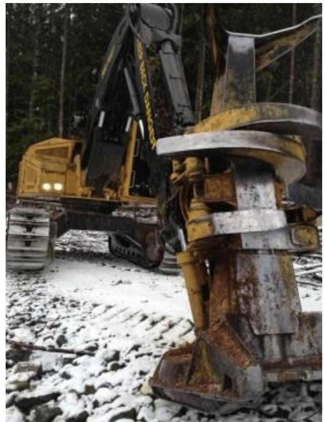
**Figure 7: Tigercat feller buncher with disk saw and accumulator**
