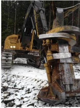
Figure 7: Tigercat feller buncher with disk saw and accumulator
