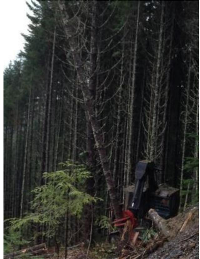
**Figure 11: Timber King self-levelling feller buncher operating on steep slope.**
