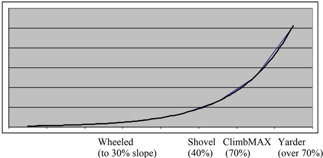
**Figure 12: Continuum of logging systems with increasing slope**
