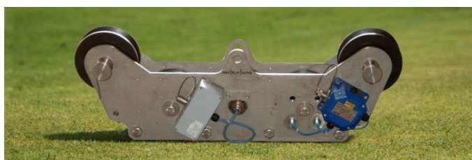
Figure 5: Scotload running-line monitor which measures tension, rope speed and distance.
