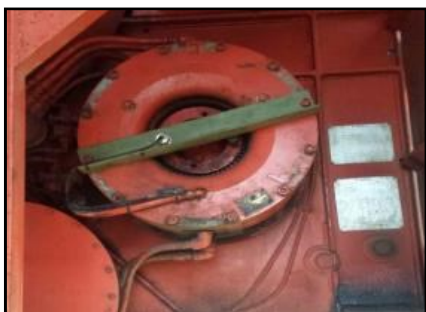
Figure 2: Proximity switch or sensor mounting for a counter. (Photo: Bill Winmill)
