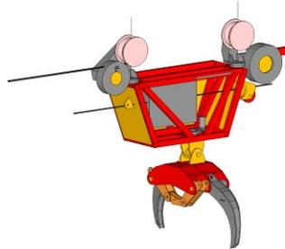
**Figure 2: Concept drawing of grapple carriage with tyre-drive mechanism**
