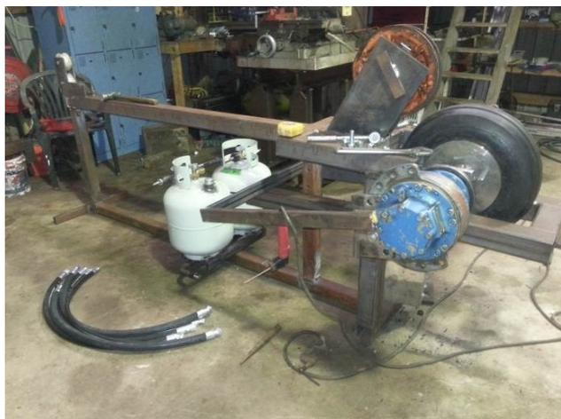
**Figure 7: Dynamometer test jig being built**
