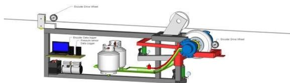
**Figure 6: Sketch-up design of dynamic test jig**
