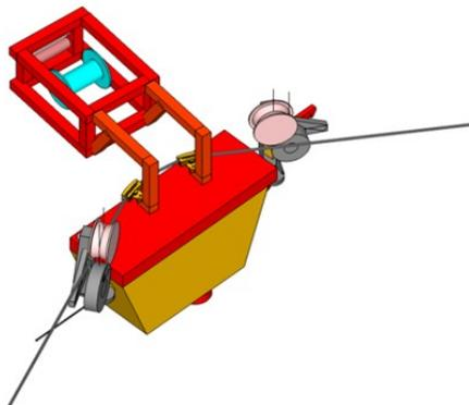
**Figure 4: The lateral yarding carriage concept showing the grapple carriage traversing past it**
