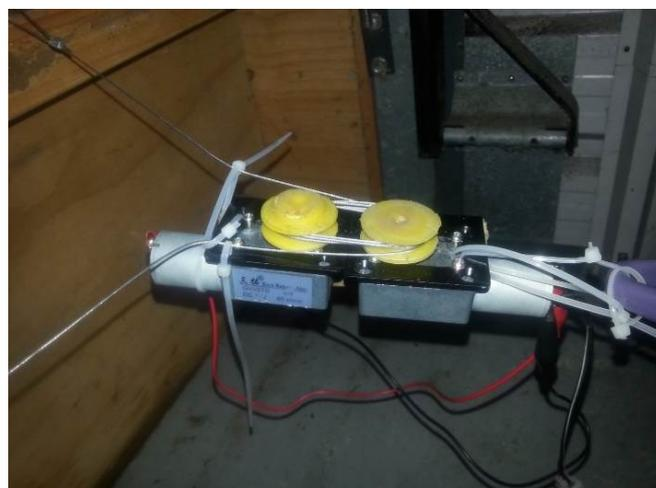
**Figure 9: A 1/20<sup>th</sup> scale model of twin capstan system**
