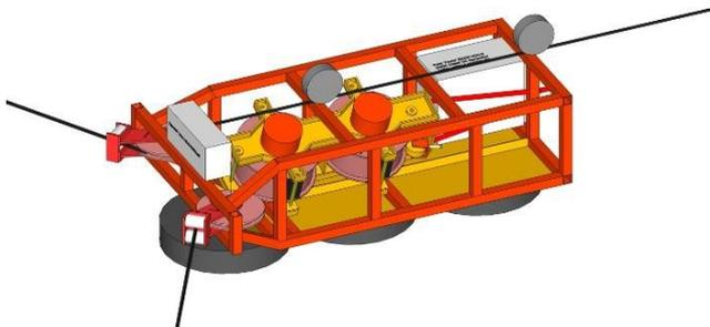
**Figure 3: Mobile Tail Hold carriage with twin capstan winches**
