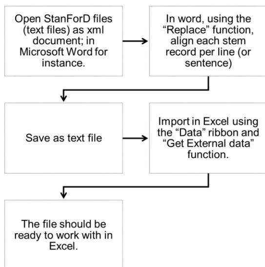
**Figure 1: Sample process for extracting data from StanForD files**
