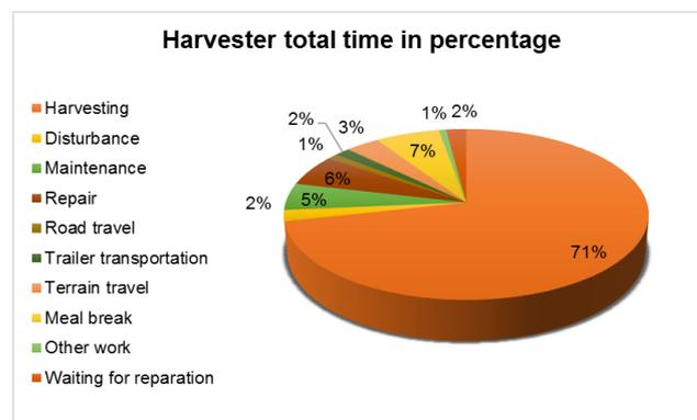
**Figure 2: Proportion of time for the various activities performed by the harvester.**
