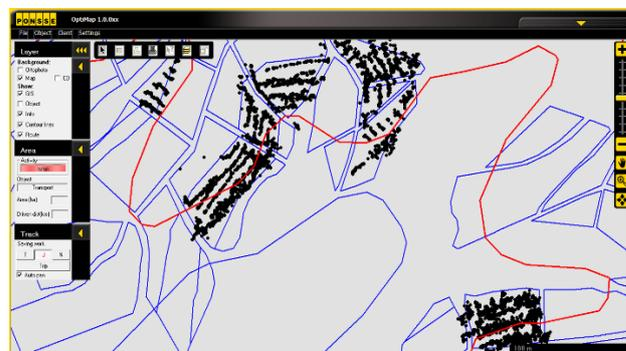
**Figure 3: Screenshot of OptiMap (Ponsse) navigation software showing layer information display. The points represent tree records, red lines are contour lines, blue polygons are stand boundaries.**
