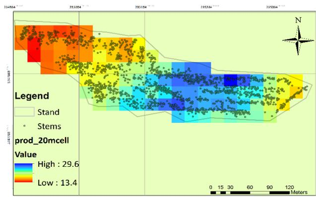
**Figure 6: Stand map where points represent individual trees and the colour of each square represents the productivity in m<sup>3</sup> from low volume (red), to moderate volume (yellow) to high volume (blue).**
