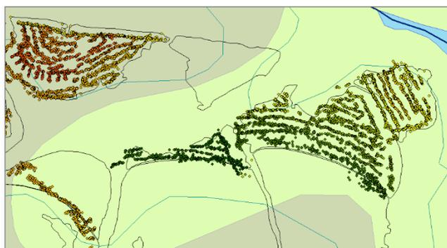
**Figure 4: Harvester machine tracks plotted on ArcGIS overlaid on stand and soil maps. Red represents the start of activity, yellow intermediate stages and green last registers.**
