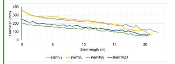
Figure 7: Profile of four stems plotted in Excel from stm files
