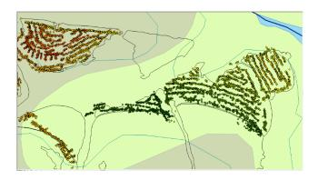
Figure 4: Harvester machine tracks plotted on ArcGIS overlaid on stand and soil maps. Red represents the start of activity, yellow intermediate stages and green last registers.
