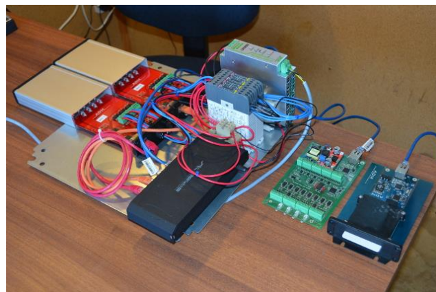
Figure 3: Internals of machine-side electronics
