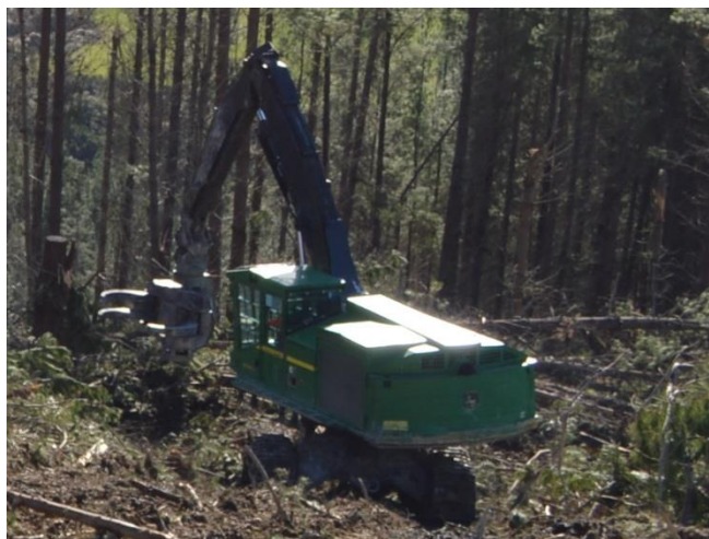
Figure 1: The John Deere 909 feller buncher
