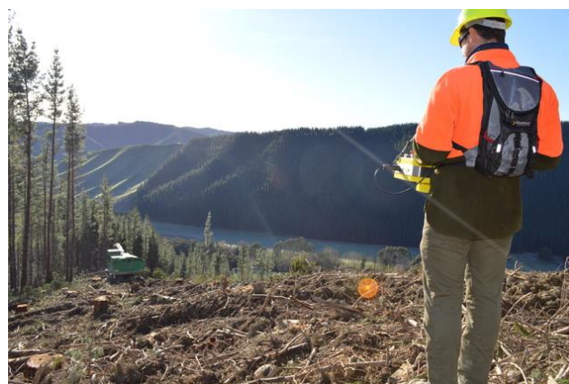
Figure 4: Ben Lewis of Wood Contracting Nelson remotely operates the John Deere 909
