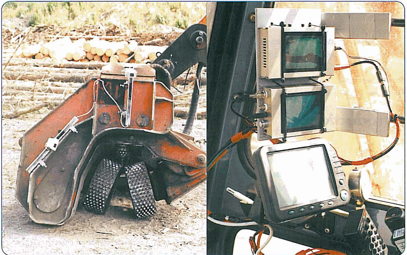
Figure 1 - Two cameras mounted on the harvester head. Images were displayed on two black and white screens within the machine cab
