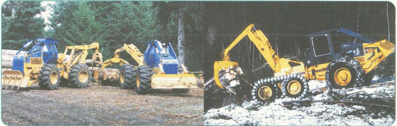
Figure 1 - SX704 Dual-arch grapple, SX704 Swing-boom grapple, SX706 double bogie Swing boom
