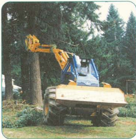
Figure 2 - SX704 skidder with attached slasher
