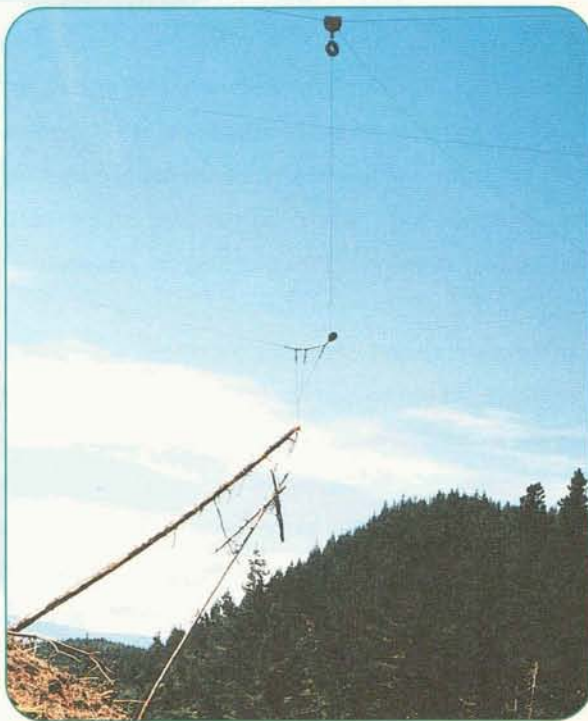
Figure 1 - A drag comprising butt and top pieces
