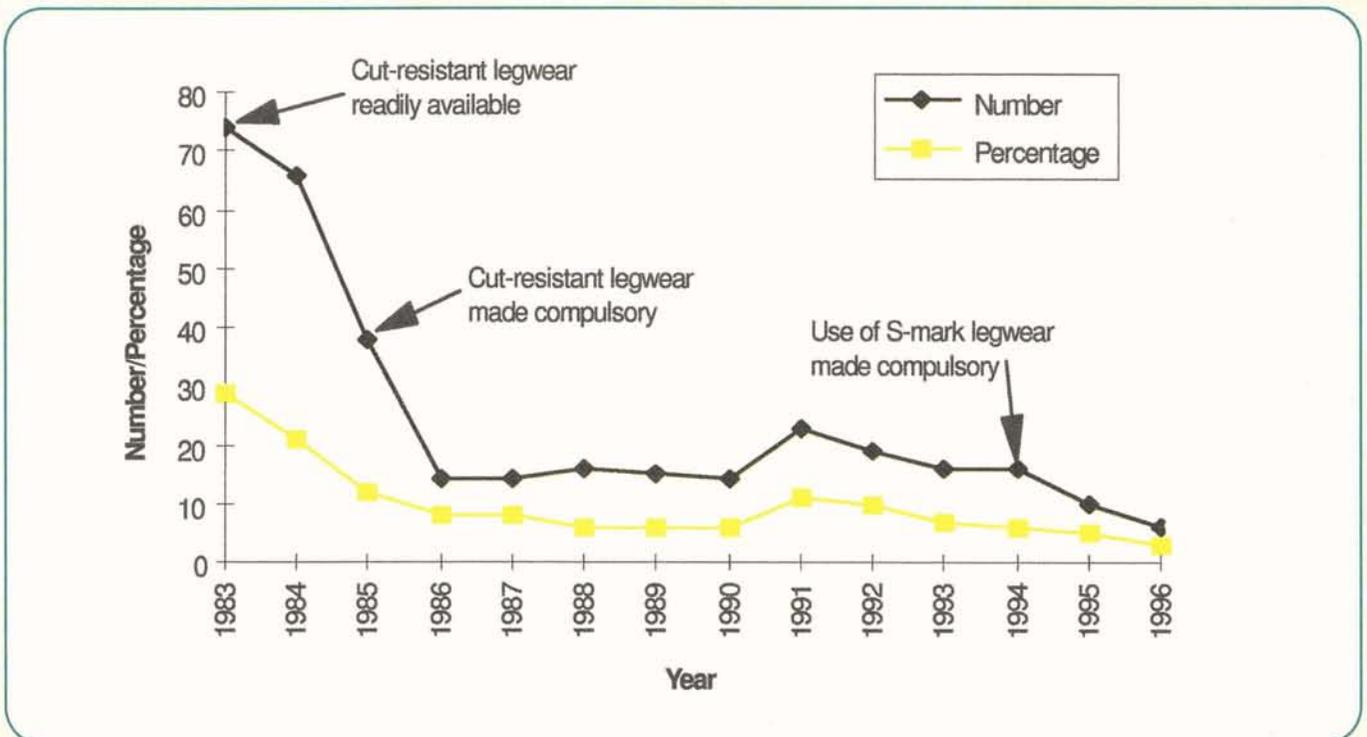
Figure 2 - Chainsaw cuts to the leg - 1983 to 1996
