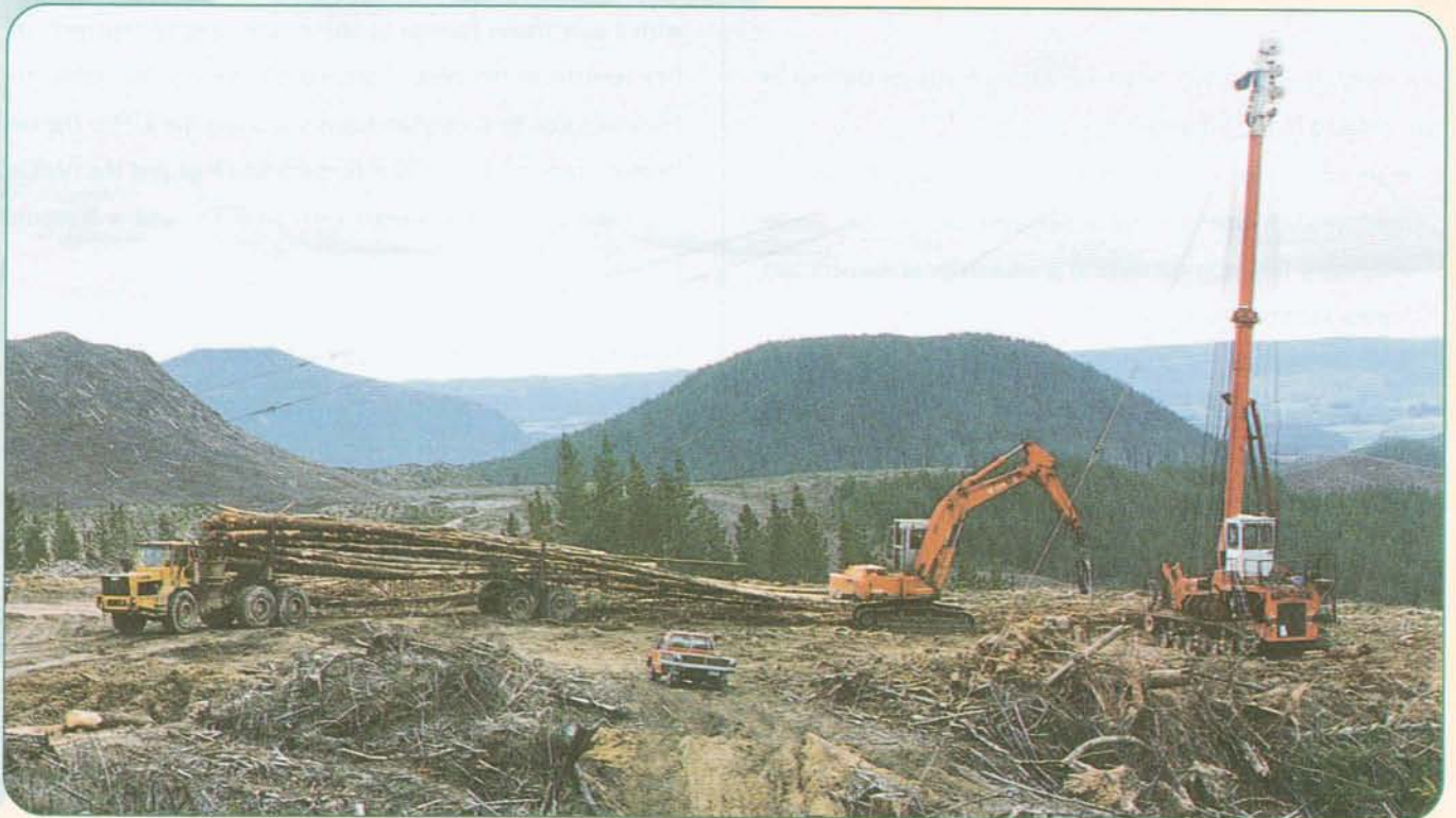
Figure 1 - Bell truck carrying full tree length logs from a hauler pad
