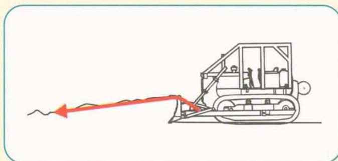
Figure 6 - This method provides little benefit over attaching the load-line directly to the blade
