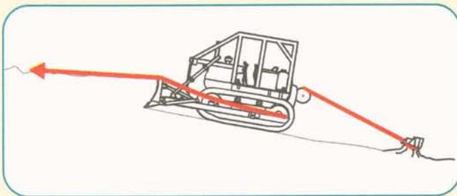
Figure 8 - Tractor winch rope tied back to a stump
