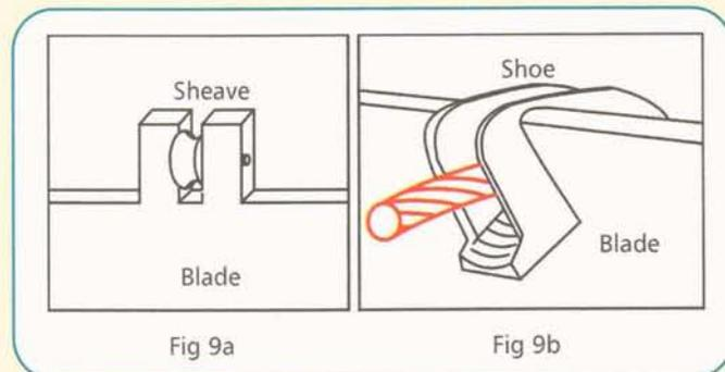
Figure 9 - Two blade - mounted fixtures to accommodate rope
