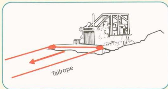
Figure 11 - Blocks hung on both corners of the blade (running skyline system)
