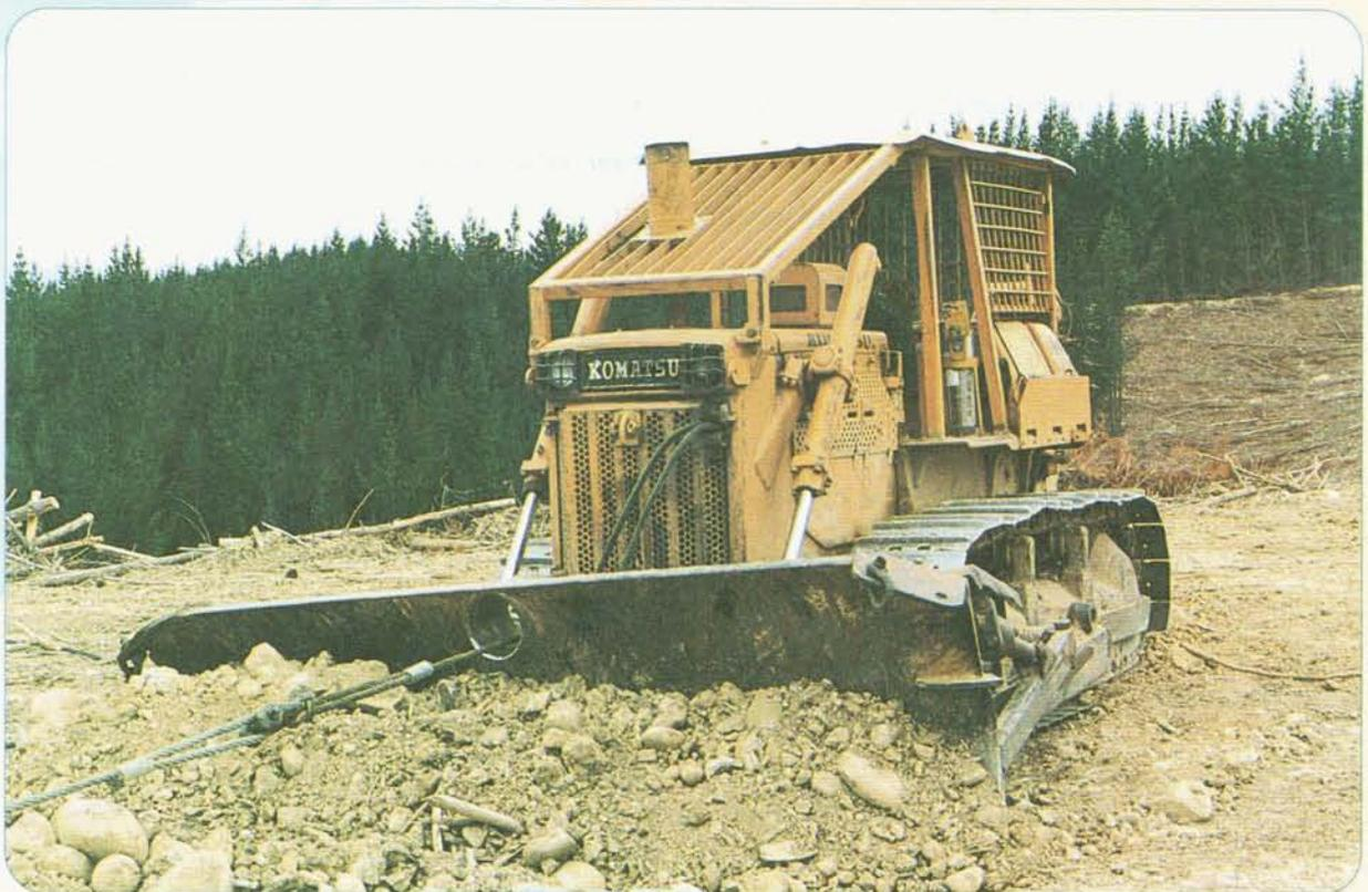
Figure 1 - Tractor mobile anchor
