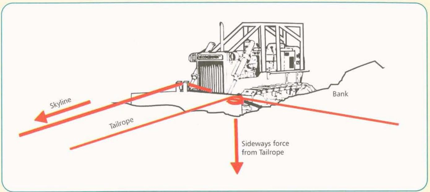
Figure 7 - Solid earth in front and beside the tractor preventing the tractor from moving forward or twisting sideways
