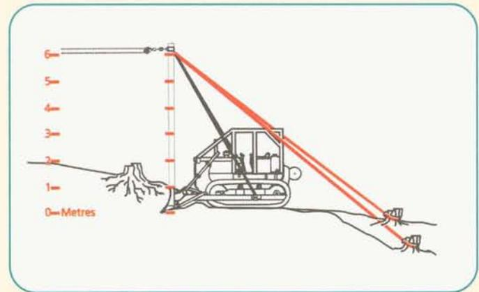
Figure 3 - Guylines attached to top of spar and anchored back to stumps
