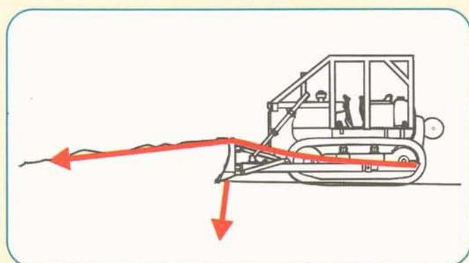
Figure 5 - The load-line puts a downward pressure on the blade proportionate to the tension
