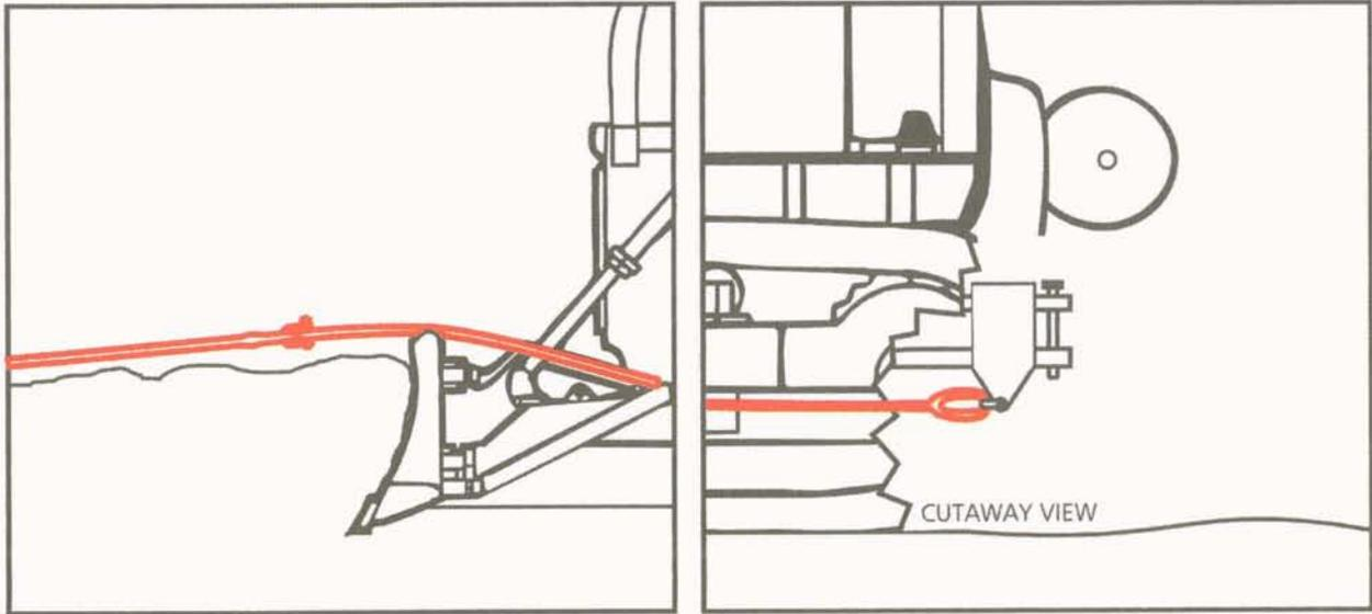
Figure 10 - Draw-bar attachment accommodating the load-line with a straight line of pull under the tractor.
