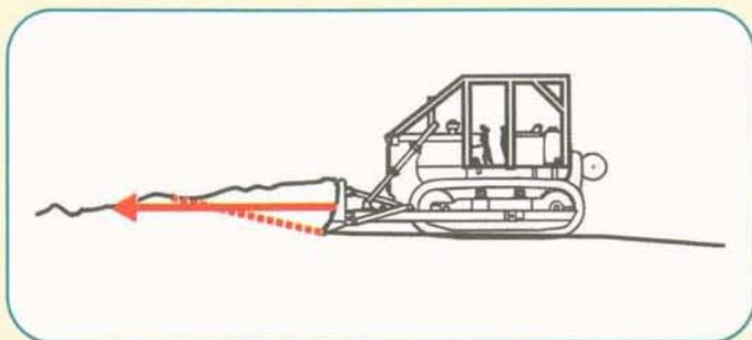
Figure 4 - Failure of the soil structure anchoring the tractor
