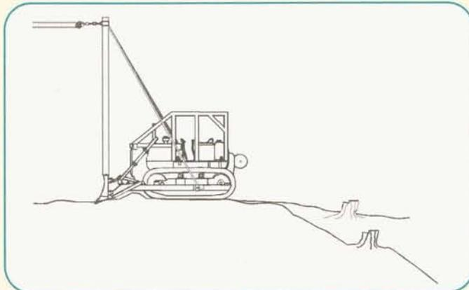
Figure 2 - Spar mounted on the blade of a tractor to help increase deflection
