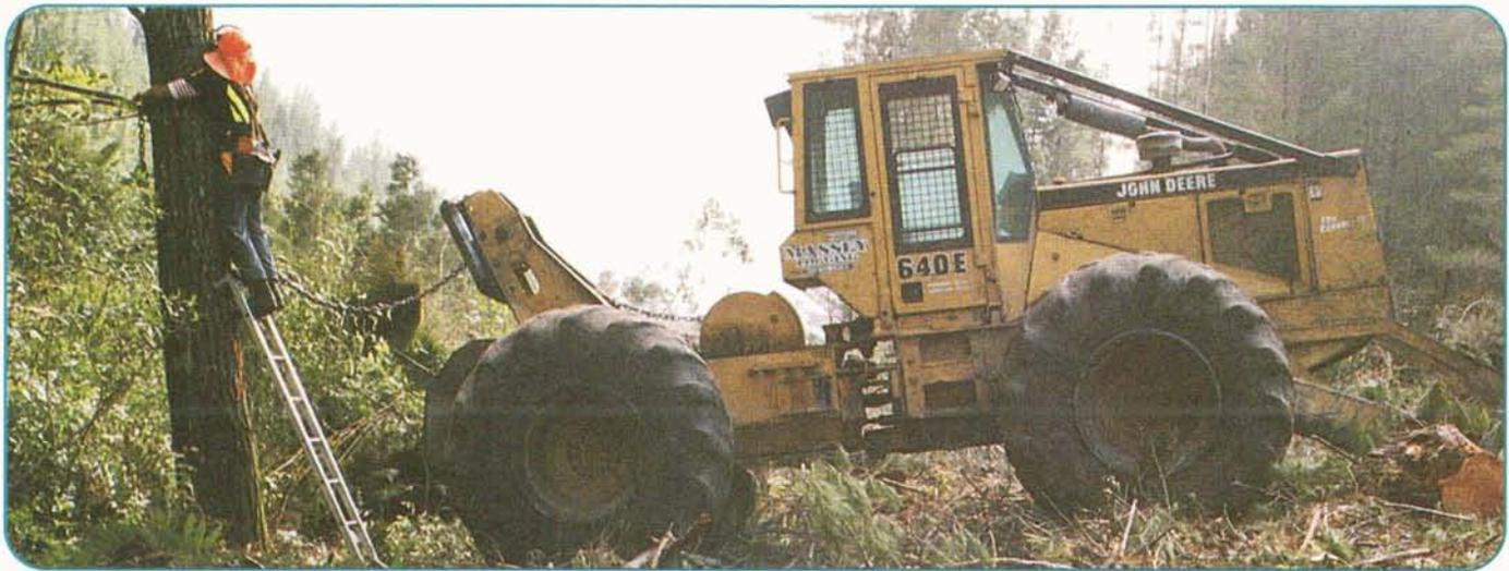
Figure 2 - Skidder-assisted streamside felling
