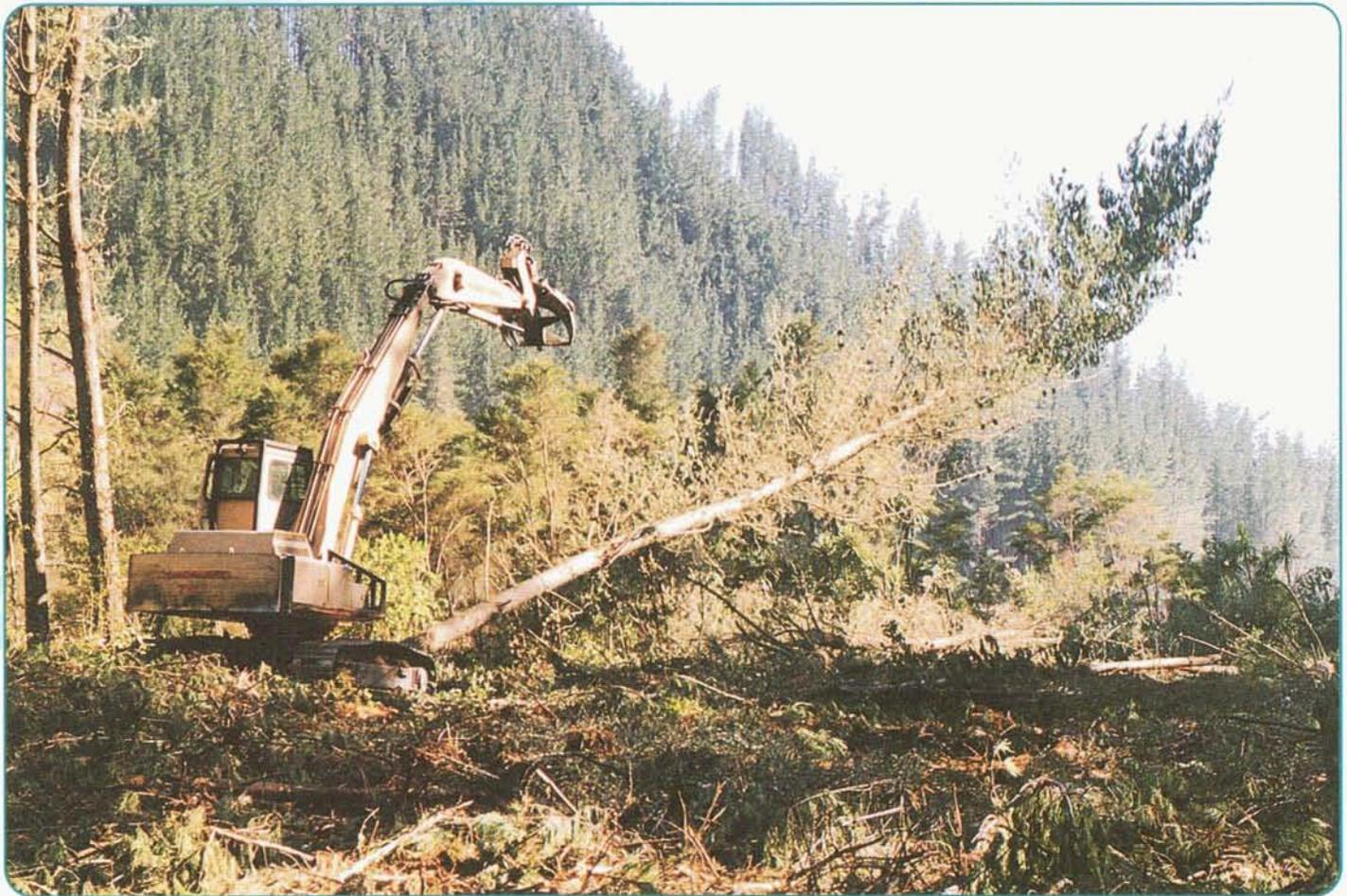
*Figure 1 - Excavator - assisted streamside felling*
