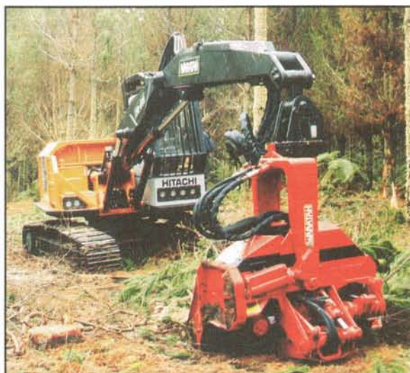
Figure 1 - Harvester and forwarder used in the mechanised thinning operation
