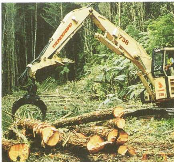
Figure 7 - Residual branching on bunched butt pieces
