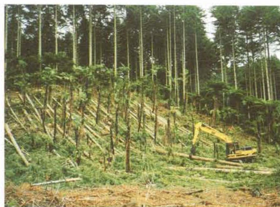
Figure 2 - Excavator bunching in Douglas Fir
