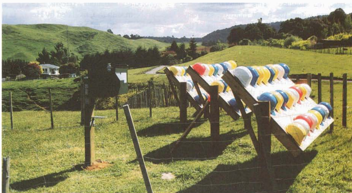
Figure 1 - Helmet exposure boards and climate monitoring station
