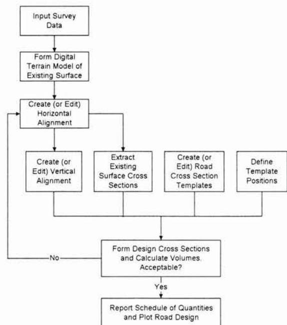
Figure 2 - Road design process using professional surveying and engineering software
