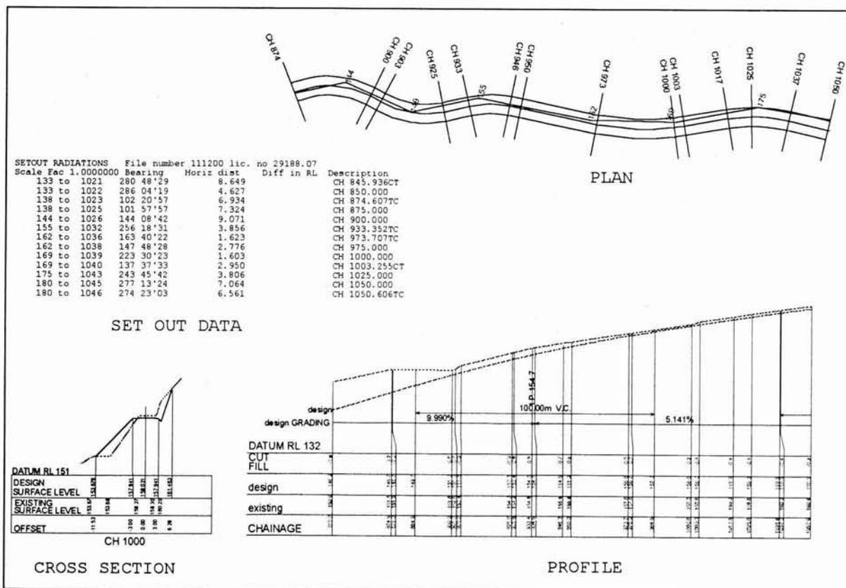
Figure 1 - Plot of plan, profile and set out data produced in GEOCOMP
