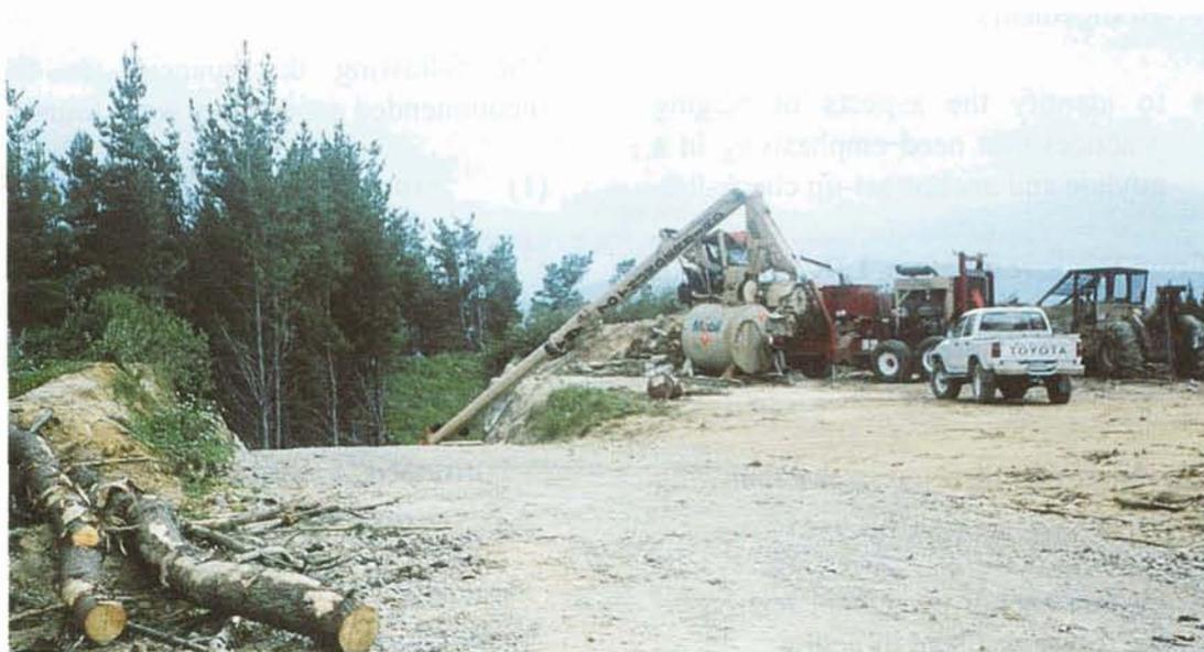
Figure 1 - Tower collapse because of inadequate guyline placement
