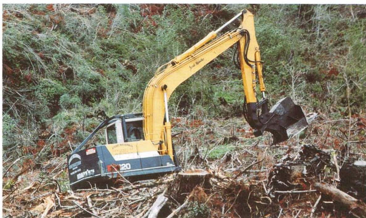
Figure 1 - The Scrub Muncher mounted on a PC120 excavator treating heavy slash and undergrowth
