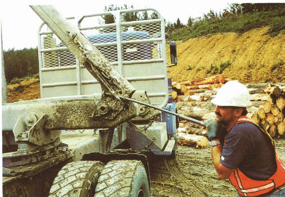
Figure 1 - Spring-assisted bolster arm
